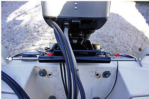
Figure 10 – Vérin installé
